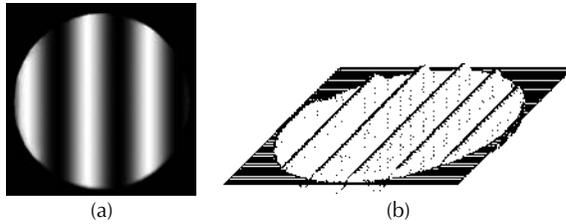
**Figure 5.25** Detection of phase error by the presence of a corrugated wavefront: (a) interferogram, and (b) wavefront.
