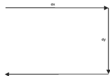
Fig. 6. Subpixel scanning trajectory to increase the image resolution by a factor of 2.
