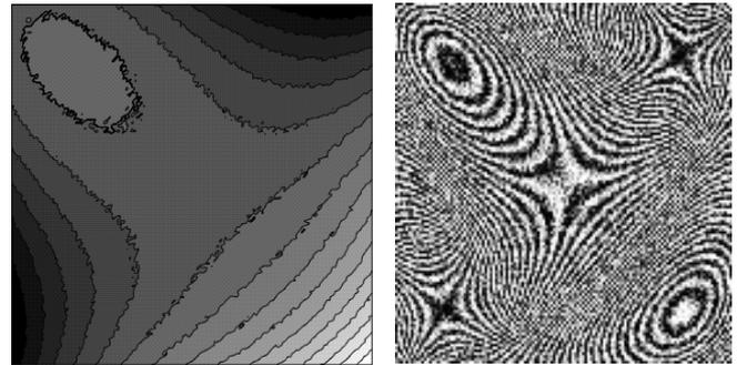
Fig. 1. Effect of spatial sampling of the field of brightness of the interferogram registered with the flat wave basic front at big curvature of the object wave front.
